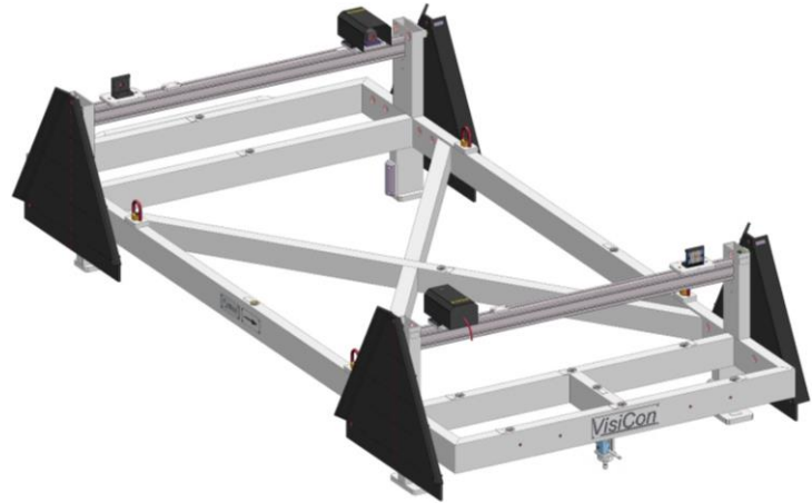
Example with targets for measurement probes and 2 lasers
