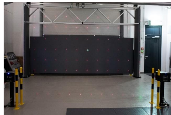
Projection of the calibration points on the projection panel of the VisiLaserWall+
