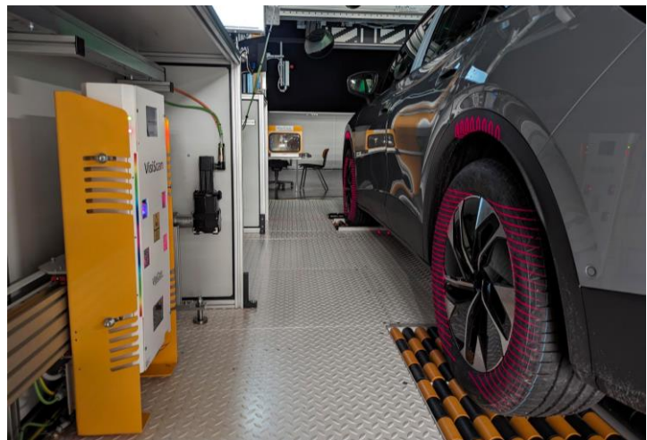
VisiScan laser lines on tire
